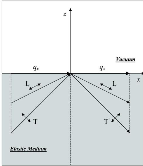
FIG. 1. The boundary between the elastic medium ( $z < 0$ ) and the adjacent vacuum medium ( $z > 0$ ). Here  $q_x$  is the common wave vector  $x$  component and the subscripts  $L$  and  $T$  mean longitudinal and transverse modes, respectively.
